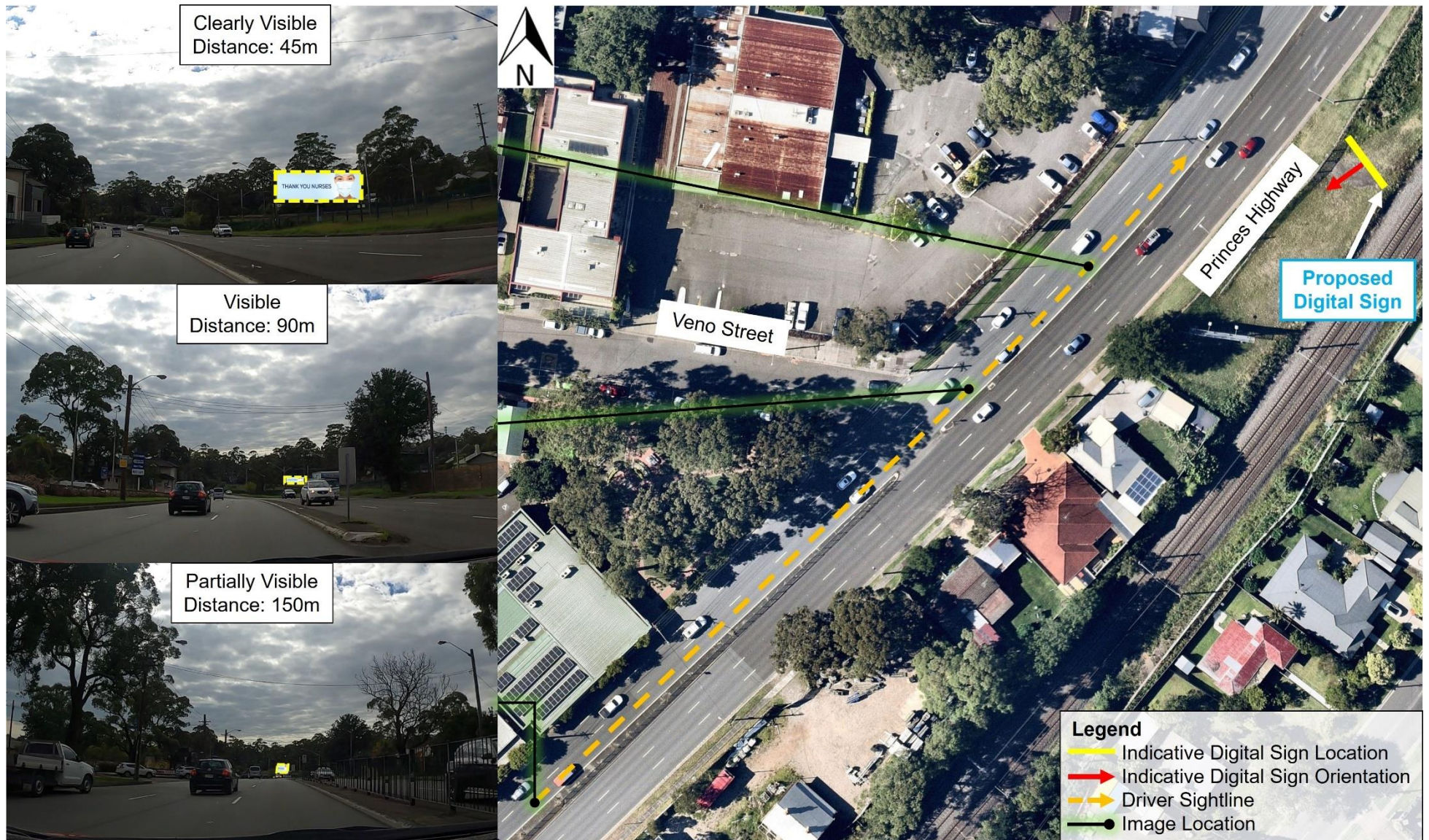
Figure 5.1: In-vehicle sightlines along the Princes Highway northbound
